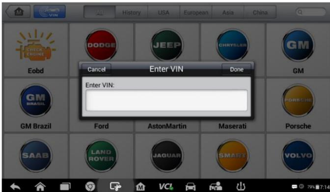
**Figure 4-6 Sample Manual VIN Input Screen**
