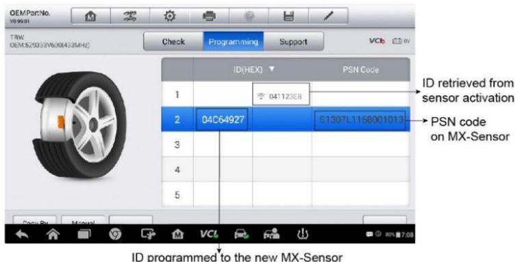
**Figure 5-34 Sample Programming Screen via OEM Part No.**
