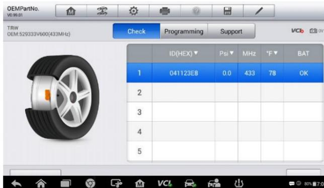
**Figure 5-33 Sample Check Screen via OEM Part No.**
